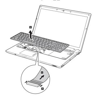
When installing: Make sure that the FPC connector is attached firmly and then lock the FPC connector.
